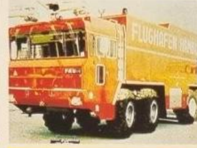
Airport Crash Tender 18 Kronenburg Tank, mounted on Faun chassis carries 18000 l water and 2000 l foam.
