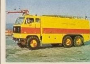
Airport Fire Crashes FCT 689 Volvo F 89 6x6 chassis and skuteng tank carrying 8000 l water and 800 l foam.
