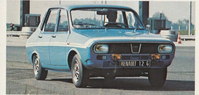
Renault 12 Gordini 4 Zylinder Reihenmotor 1,565 Liter 113 PS (DIN), 125 PS (SAE), 83,2 kW
